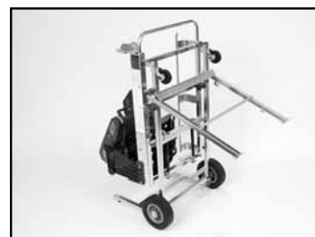
(F) Tilt Saw backwards to upright position.
