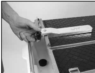
(B) Set the Adjustable Cutting Guide to cut a 1/16-inch strip.
