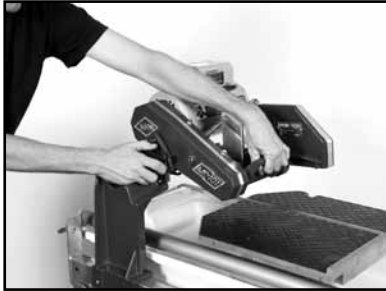
(A) Loosen Cutting Head Adjusting Knob.
