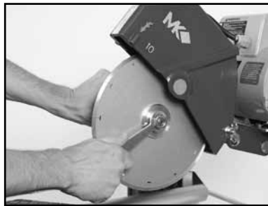
(B) Remove Retaining Nut and Outer Flange, depress and hold the Shaft Lock push button and loosen.
