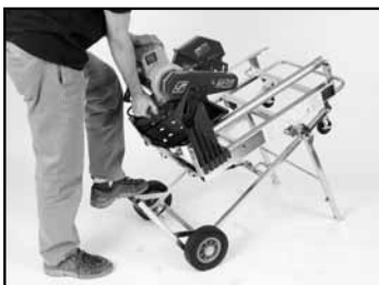
(G) Lift saw up vertically with Cutting Head Handle.
