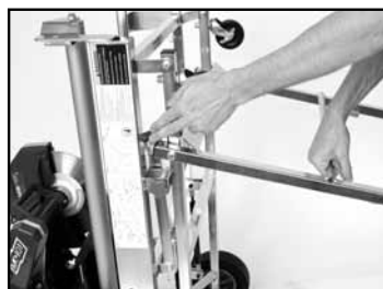
(G) Hold up Front Legs, flip and hold Red Leg Lock to unlock Front Legs.
