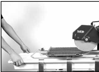
(A) Remove Water Pan.
