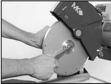
(A) Remove the Diamond Blade.
