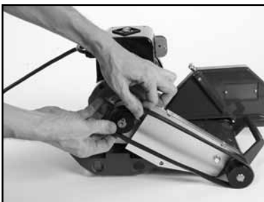
(K) Install the new belt (MK Diamond Part No. 158194).
