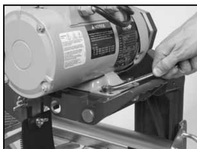
(P) Tighten the motor mounting bolts.
