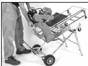
(E) Push down on Cutting Head Handle to collapse the saw.
