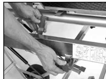
(C) Release Green Knob to secure Safety Arm.
