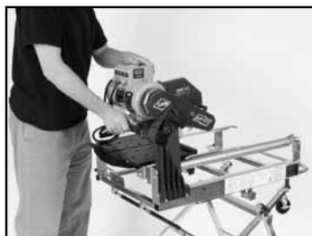
(H) Push down lightly on Cutting Head Handle to ensure saw is fully supported.
