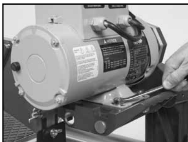
(G) Loosen the motor mounting bolts, if re-tensioning only go to step N.
