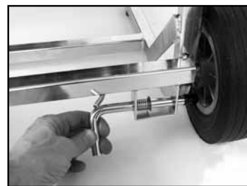
(I) Pull back pin and place behind retaining rod to unlock wheel.
