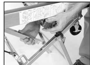
(I) Pull Green Knob to release Safety Arm.
