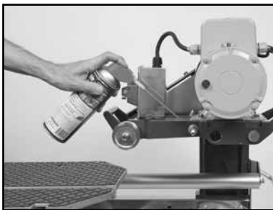
(H) Lubricate the Blade Guard Pivot Shaft.
