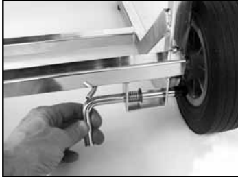
(A) Pull, turn & release pin to lock Wheel.
