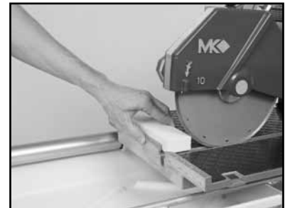
(C) Position the Dressing Stick. Cut the Dressing Stick 7 or 8 times to dress the Blade.
