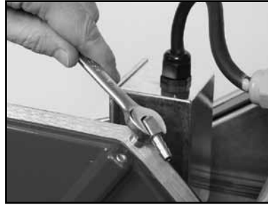
(E) Remove the Blade Guard Intake Fitting. Go to Step J.
