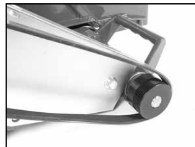
(L) Verify the belt is seated in the grooves of both pulleys.
