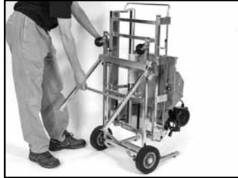
(B) Stand on left side of saw. Pull Blue Knob and pull Front Legs out slowly.
