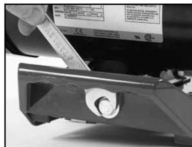
(H) Loosen the Motor Adjustment Strap.
