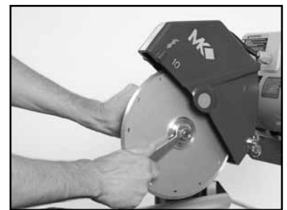
(F) Install Retaining Nut and Outer Flange, depress and hold the Shaft Lock push button and tighten.
