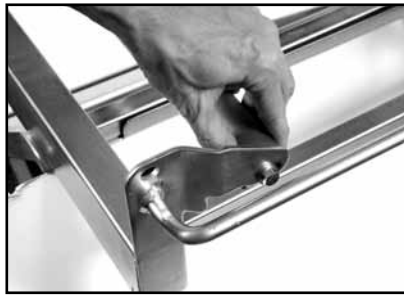
(E) Move Guide Bar until Square rests evenly across Blade.
