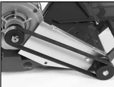
(E) Inspect the belt for cracks, fraying, separation and wear. Go to step H if replacement required.
