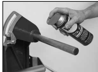
(L) Lubricate the Cutting Head Pivot Shaft.
