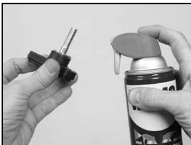
(J) Lubricate the Cutting Head Adjustment Knob.
