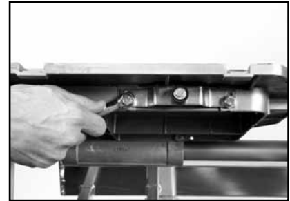
(F) After Squaring, tighten Movable Cutting Table Wheel Assembly.
