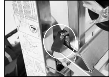
(C) Pull legs until they are locked by Red Leg Lock.
