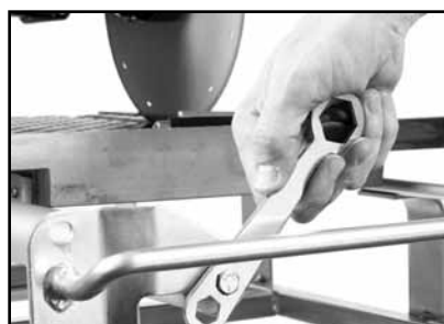
(B) Tighten Guide Bar Retaining Bolts.
