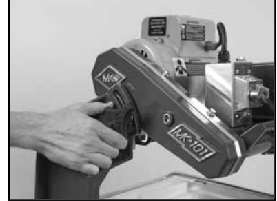
(C) Tighten the Adjusting Knob.
