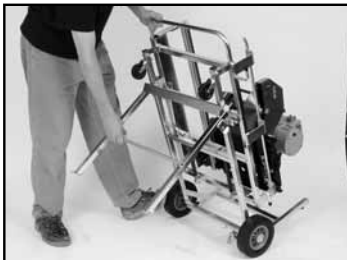
(D) Place left foot on left wheel, left hand on Handle and right hand on Front Legs.
