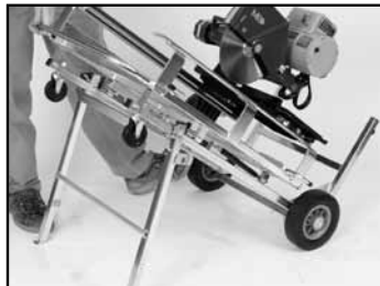
(E) Tilt Saw forward and rest Front Legs on ground.
