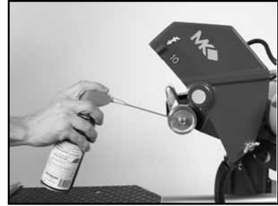
(C) Lubricate the Arbor Shaft.
