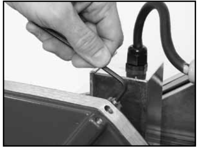
(F) Remove the Cooling Channel cover screws.
