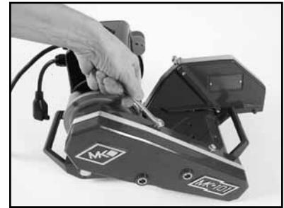
(C) Remove the Belt Guard. Loosen the two top bolts.
