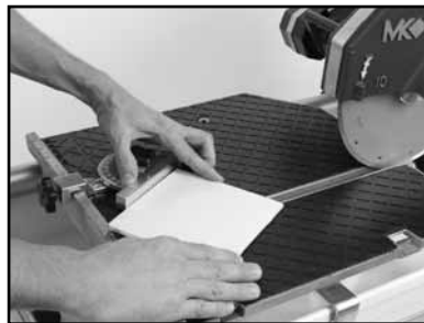
(D) Position the tile against the 90° Protractor and the Ruler/Stop. Turn the motor ON.
