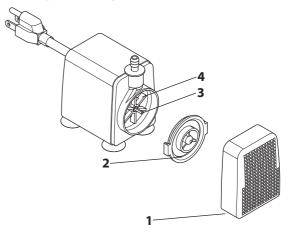
A cloth may be used to remove iron particles that might adhere to the magnetic rotor shaft.
