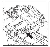
Make sure that the cutting blade can rotate freely until it is completely stopped.
