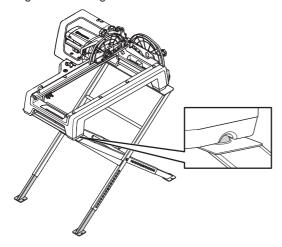
Use the two clamps, one on each side, to fasten the frame on to the stand.
