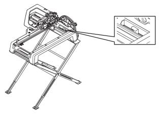
The machine can also be used without frame legs or placed on a workbench. · Pull out the locking knob on the conveyor cart.
