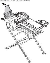
• With a push, the slurry collector tray can be locked in its inner position.
