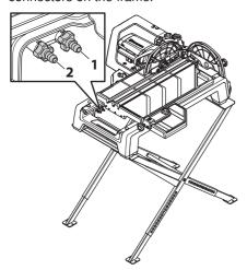
Place the water pump in the water tray. The pump compartment should face towards the working position. Slide in the water tray.
