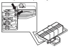
Screw the cutting guide onto the conveyor cart. The guide can be folded outwards for angled cuts. Use the angle markings on the cutting guide to set the correct angle.
