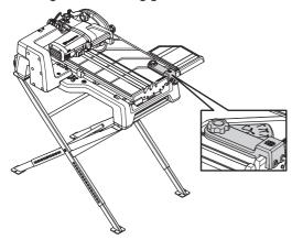
Assemble the water recovery tray. Make sure that the plastic hook grips the metal bar under the cart.
