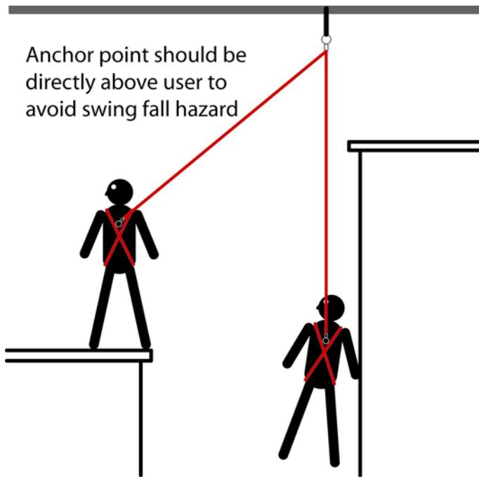
Be sure to consider Swing-Fall when calculating your Clear-Fall requirements and checking the fall path for hazards and instructions. Failure to do so may result in serious injury or death. Should you have any questions regarding Free-Fall, Clear-Fall, Swing-Fall or other hazards in the fall path, be sure to contact *FallTech* or consult with a competent person or your direct supervisor on your job-site.
