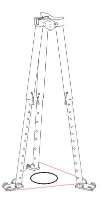
The FallTech 7275 Tripod is intended to provide a portable anchorage mount for the mounting of lifeline components of a comprehensive confined space entry, retrieval and rescue system. It should be erected above the opening of the confined space. It will accommodate round openings up to 5 feet in diameter and up to 4 feet square openings.
