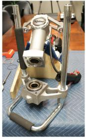
Separate the lower body from the upper driver body and slide the throttle off the end of the handle. Remove the gasket and sleeve o-ring from the lower body and discard them.
