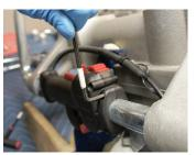
Loosen slightly (do not remove) 2 hex bolts on opposite corners of the throttle with a 5/32" hex key (4mm) just enough to allow it to slide freely on the handle tube.
