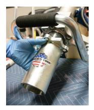
Place lock washers (300750-4), over the chuck bolts (300717-4) and apply Loctite 7649 Primer N to threads of each chuck bolt and to chuck bolt holes on the lower body and allow them to dry. When dry, apply Loctite 243 thread locker to threads of bolt holes.
