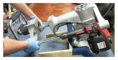
Set out the lower body bolts (300702-4 or 300701-4) and apply Loctite 7649 N Primer to threads of each bolt and to bolt holes on the upper body and allow them to dry. When it has dried apply Loctite 243 thread locker to bolt holes on the bottom of the upper driver body.
