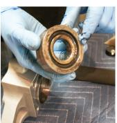
Remove the entire anvil o-ring cup with contents intact from the lower body.
