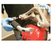
the throttle into a center position and tighten the hex nuts with a 5/32" (4mm) hex key. Set out the top handle bolts and apply Loctite 7649 Primer N to threads of each bolt and to bolt holes on the handles followed by an application of Loctite 243 thread locker to bolt holes on top of side handles. Using acetone or solvent, clean and springs and inside of handle collars, then apply grease to both.
