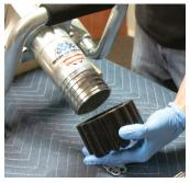
Removing the Existing Chuck
