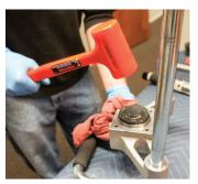
Stand the handles and lower body in the upright position. Insert the lubed anvil with o-ring into the lower body. If it does not seat completely, tap it lightly with a soft mallet to seat in proper position. It may be a tight fit.
