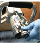
Then using a 1/4" hex drive bit remove the 4 chuck bolts and 4 lock washers and detach the chuck.
