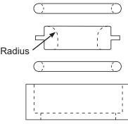
If the elements in the anvil o-ring cup need to be reassembled, do so in this order: 1.) lower o-ring; 2.) large retainer with radius to the top; 3.) top o-ring. Then insert assembled anvil o-ring cup into the lower body.
