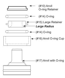
Insert O-ring into Anvil O-ring Cup, then insert Large Retainer (with large radius at bottom towards the anvil), then insert other O-ring.
