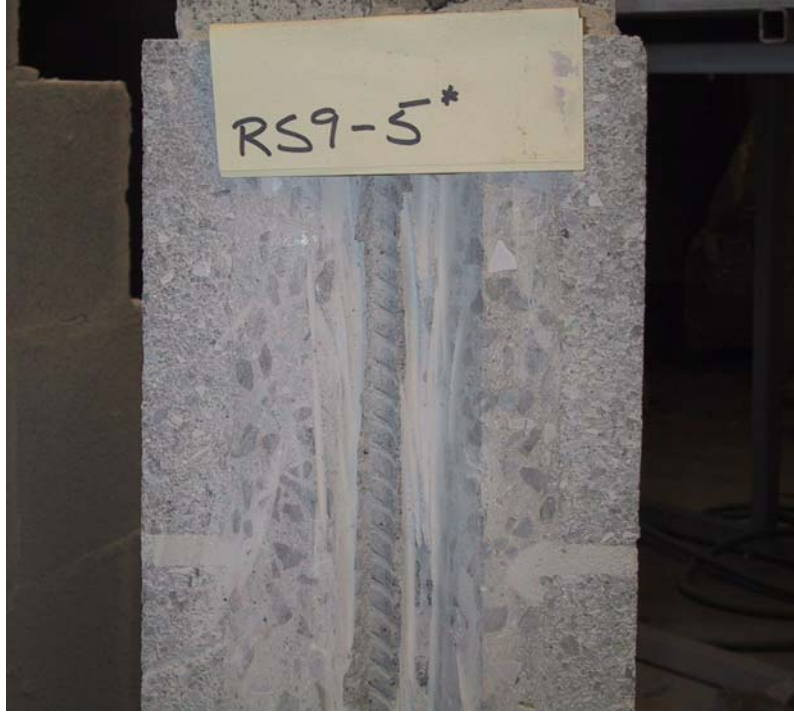
Figure 7. Wall cross-section with Oztec Rebar Shaker consolidation
