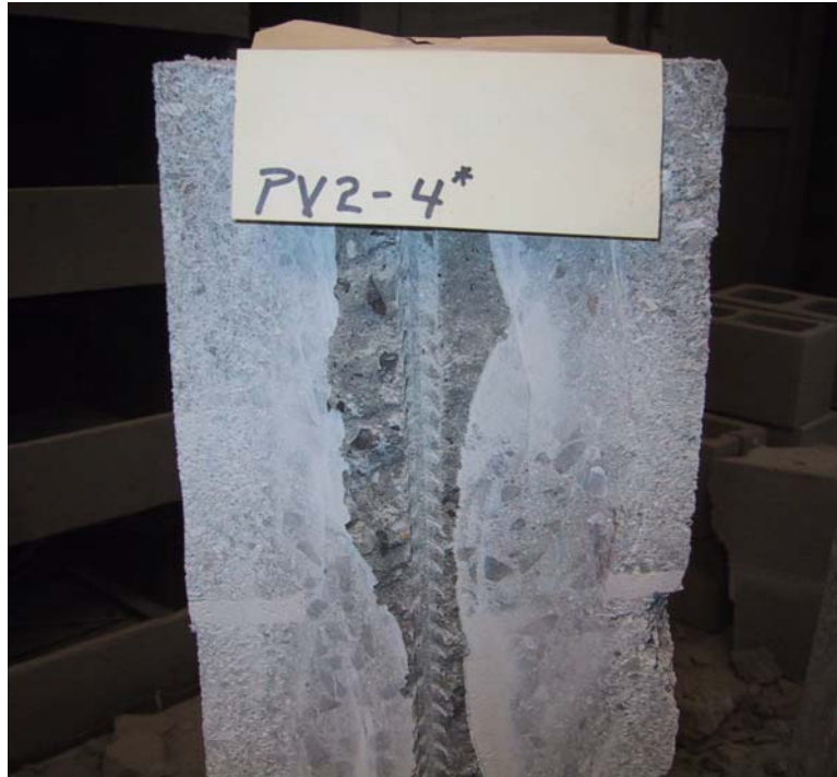
Figure 5. Wall cross-section with pencil vibrator consolidation
