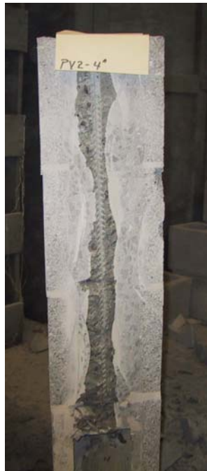
Figure 4. Wall cross-section with pencil vibrator consolidation
