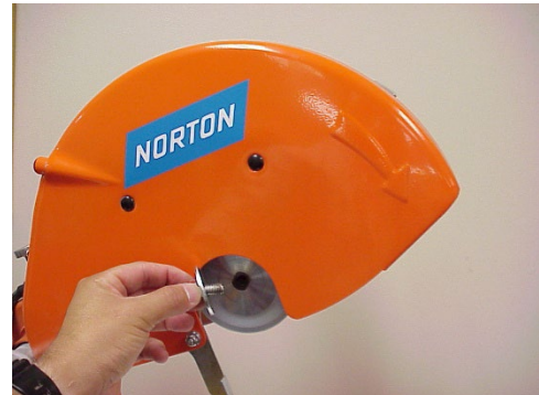
Blade Shaft Bolt Removal
