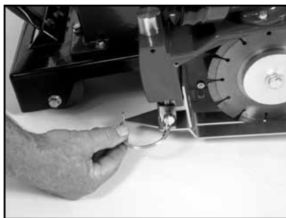
(B) Insert pin through Skid Plate and rear plunger.
