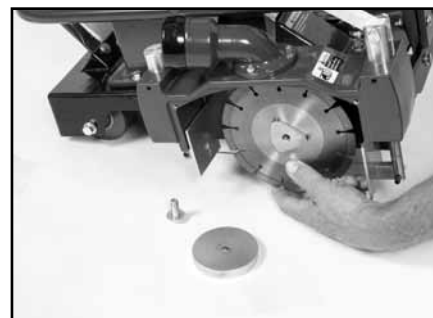
(C) Remove the Blade Nut and Outer Flange.
