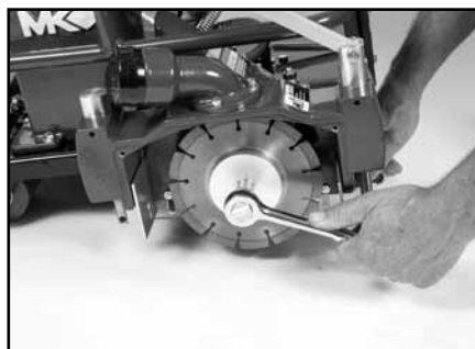
(B) Loosen the Blade Shaft Nut while holding the Shaft Wrench steady.
