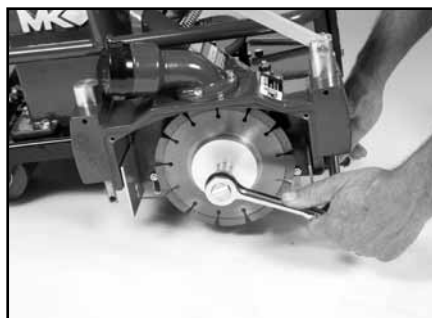
(E) Install the Outer Flange and Blade Shaft Nut. Tighten Blade Shaft Nut holding the Blade Shaft steady.
