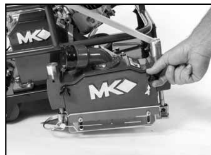
(F) Replace the Blade Guard and tighten Blade Guard Nut.
