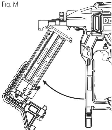
4. Remove jammed/bent staple, using pliers if necessary.
