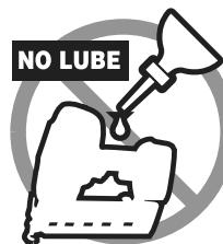
DEWALT tools are properly lubricated at the factory and are ready for use. However, it is recommended that, once a year, you take or send the tool to a certified service center for a thorough cleaning and inspection.
