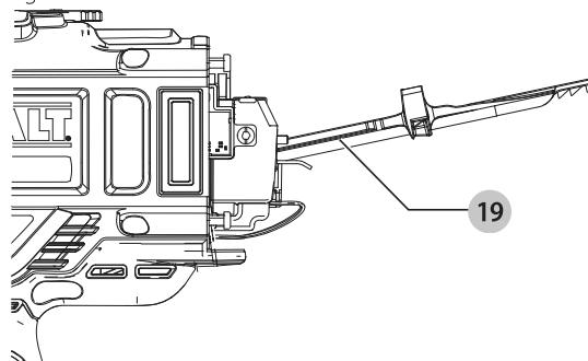
10. Return the driver, guide rods, bumpers and housing end cap back onto the unit. It is important to try the alignment of the driver and the flywheel before screwing the housing end cap back on to the unit. This can be done by connecting a battery and pushing then releasing the nose of the unit against a bench or hard surface. This will start the motor spinning.
