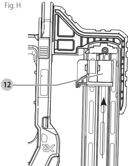
3. Drop staple strips into the loading slot of the magazine, making sure the staple heads align correctly with the slot opening. (Refer to **Staple Specifications** to determine compatible size.)
