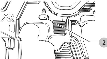
When the trigger lock-off is pressed to the left, the tool will be fully operational. The trigger lock-off should always be locked off whenever any adjustments are made or when tool is not in immediate use.
