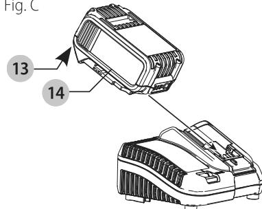
2. Insert the battery pack **14** into the charger, making sure the battery pack is fully seated in the charger. The red (charging) light will blink continuously indicating that the charging process has started.
