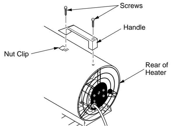
Figure 5 - Attaching Handle
