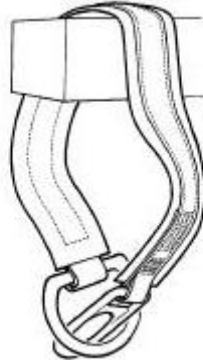
Fig. 3.4 Correct Installation of Web Pass-Thru Sling Anchor
