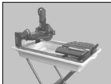
(E) Inspect the MK-370EXP Saw for damage – ensure the cord is free of cracks or cuts
