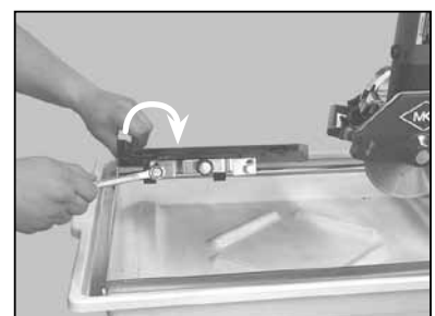
(I) Tighten Movable Cutting Table Wheel Assembly
