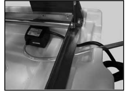
(C) Position pump as shown and place the pump electrical cord and cooling transfer tube under the frame.
