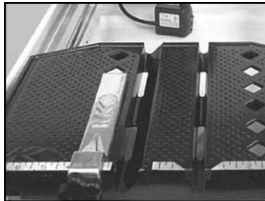
(E) Position the Adjustable Cutting Guide to desired cut length
