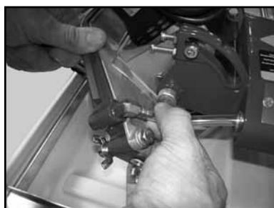
(B) Connect the Cooling Transfer Tube to the inlet connection on the Blade Guard
