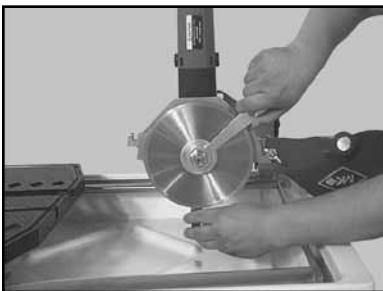
(G) Install the Retaining Nut and Outer Flange and then tighten using the Blade and Shaft Wrenches
