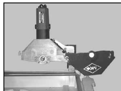
(C) Open the Blade Guard
