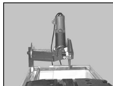
(C) Verify the Cutting Head is completely installed and seated on the Post
