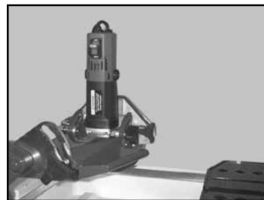
(K) Tighten the Blade Guard, Retaining Knob
