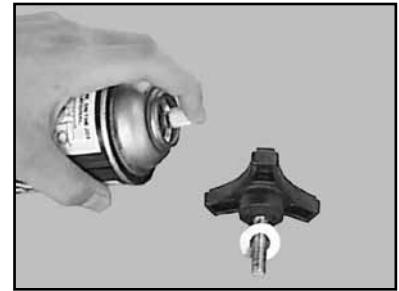
(L) Lubricate the Cutting Head Adjustment Knob
