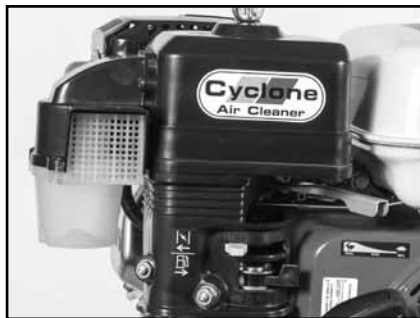
(E) Clean engine air filter. Refer to Engine Manual.
