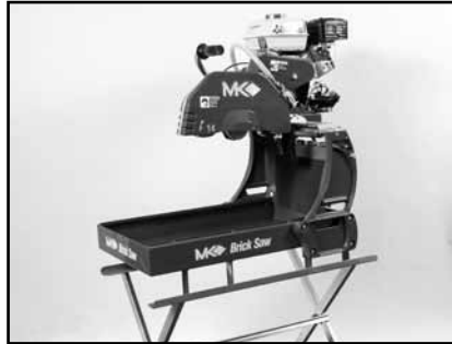
(B) Set saw on stand as shown.
