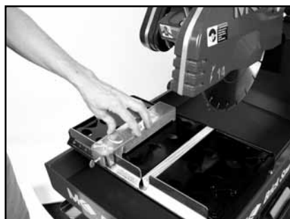
(B) Position adjustable Cutting Guide above movable Cutting Table. Align parallel slots. Seat and tighten the adjustable Cutting Guide retaining thumbscrew.
