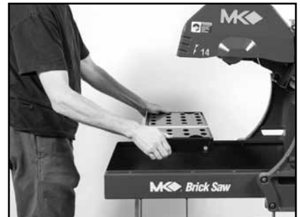
(F) Install the movable Cutting Table.
