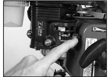
(C) Place Fuel Valve in the OFF position.
