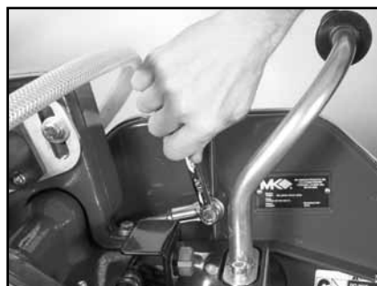
(E) Disconnect the Blade Guard Adjustment Bar.
