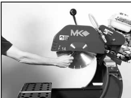
(Y) Install the Diamond Blade.
