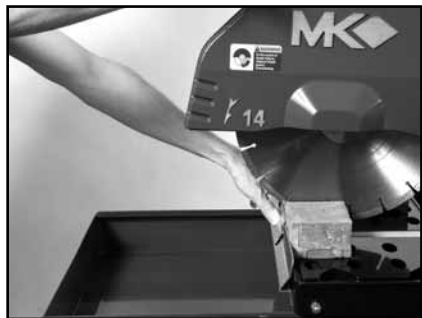
(G) Step Cut "Pull" stroke. Lower blade 1/4" - 1/2" inch.
