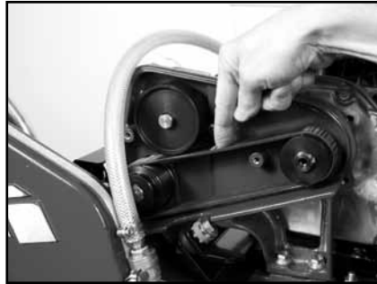
(Q) Check Micro-V Belt tension (proper tension 1/8-inch).
