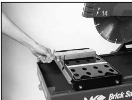
(A) Set the adjustable Cutting Guide.
