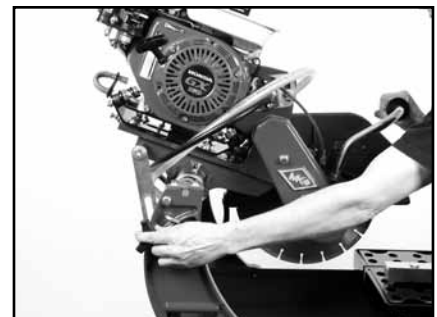
(C) Lock Cutting Head in the down position.
