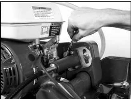
(W) Move Water Pump Pivot Plate down and retighten retaining bolts.
