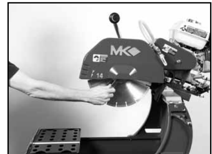
(F) Install Retaining Screw then tighten.
