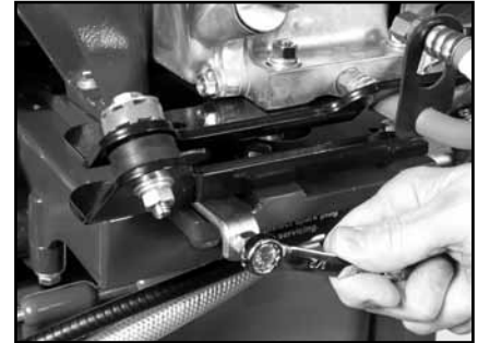
(C) Verify engine adjustment Straps are tight.
