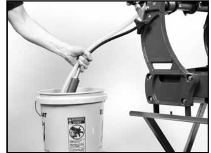
(C) Place the Water Pump Assembly into a filled Water Container.
