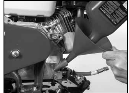
(C) Fill Oil Reservoir.
