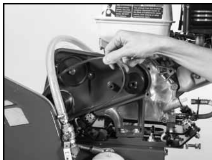
(N) Install the new Micro-V Belt (MK Diamond Part No. 156294).
