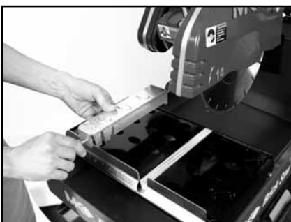
(A) Loosen adjustable Cutting Guide retaining thumbscrews by turning counter-clockwise.
