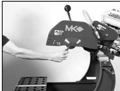
(B) Identify and remove Retaining Screw and Outer Flange
