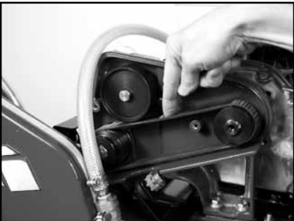
(T) Check Micro-V Belt tension (proper tension 1/8-inch).
