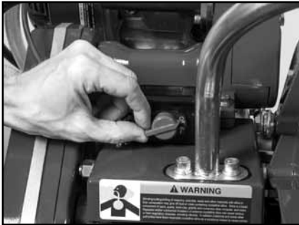
(A) Place Engine Switch in the OFF position.
