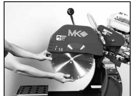
(C) Install Diamond Blade onto Blade Shaft
