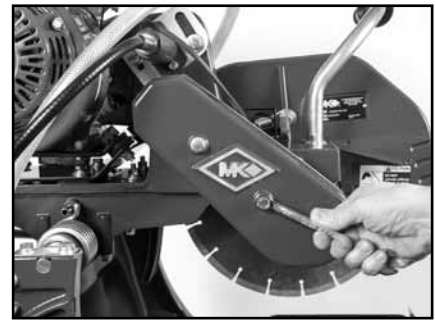
(O) Install the Belt Guard.
