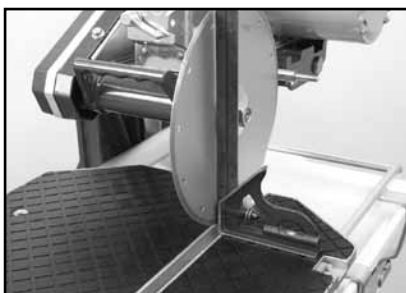
(G) Re-verify the Diamond Blade is Square to the Movable Cutting Table.
