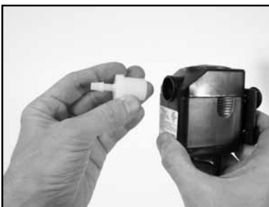
(A) Install Water Pump Discharge Fitting.
