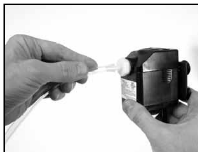
(B) Press one end of the Cooling Transfer Tube onto the Water Pump Discharge Fitting.
