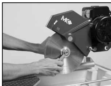
(G) Install Retaining Nut and Outer Flange, depress and hold the Shaft Lock pushbutton and tighten Retaining Nut.
