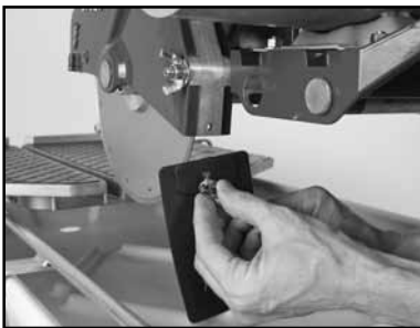
(A) Install the retaining thumbscrew through the washer and Splash Guard then align to the hole found on back of the Blade Guard.
