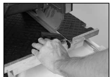
(C) Move the Cutting Table back and forth to re-verify Blade is even across all points of Square.
